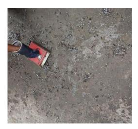
Metal scrap and non metal scrap on the shop floor is to be regularly cleaned. Metal scrap is currently cleaned by using a magnet shown above by operator. Metal/Non metal scrap chips generally have sharp edges and may injure operators or anyone who steps over it. A robot to regularly clean the shop floor is visualized. It may or may not have a battery.
