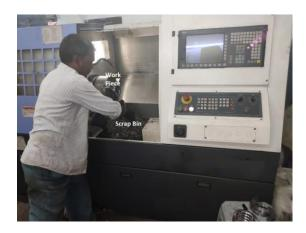
After the work piece is machined, metal scrap, usually of low carbon steels or Aluminium alloys are collected in the 'scrap bin'. Operator then manually removes the scrap from the scrap bin. As the scrap chips have sharp edges, chances of the operator's hands getting bruises are high. Hence a robot to empty the scrap bin is visualized, reducing the possibilities of injuries to the operator and improving the consistency.
